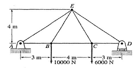
b. Determine the forces in members AC and AB of a simple triangular truss with the loading and support system shown in figure. Use the method of section.
