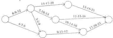
For each activity, the three estimates  $t_0$ ,  $t_m$  and  $t_p$ are given along the arrows in the  $t_0 - t_m - t_p$  order. Enter calculations in the tabular form.
