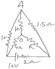
f. Using mesh analysis find the branch current in following network:
